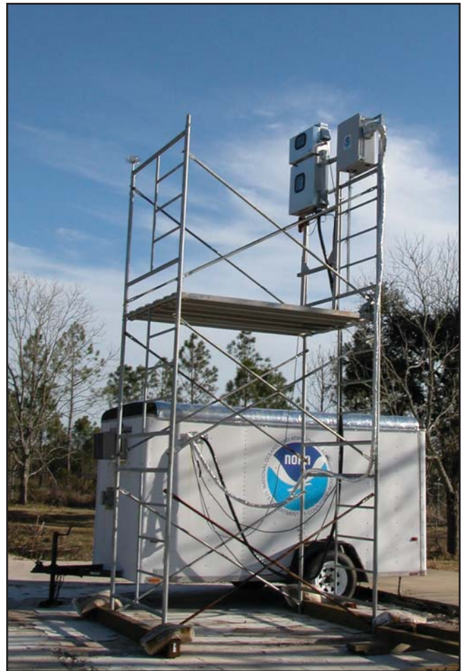
The Grand Bay NERR has partnered with the National Oceanic and Atmospheric Administration to set up a station to test for mercury in the atmosphere to learn more about its effects on coastal and aquatic ecosystems as well as human health.
