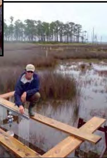
NERR staff measuring subsidence and accretion of marsh elevation at NERR, part of a broader sentinel site program to measure impacts of sea level rise in our nation's estuaries.
