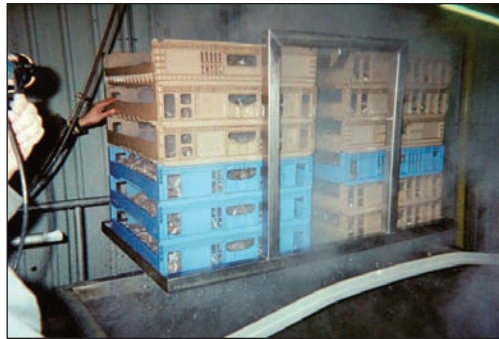
Fig. 4 Cartload of oysters is immediately cooled down to 40 degrees Fahrenheit for 15 minutes.
