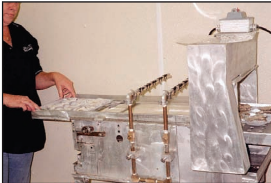
Fig. 2 Trays of half shell oysters go through the glazing machine to seal the natural juice of oysters.
