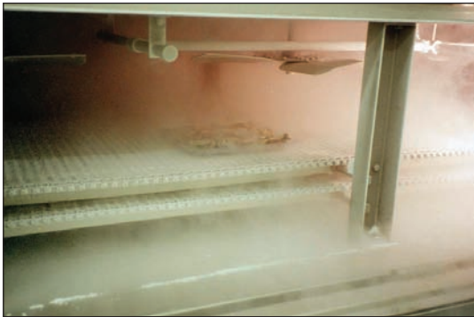
Fig. 1 Half shell oysters on a tray being frozen through the IQF machine tunnel.
