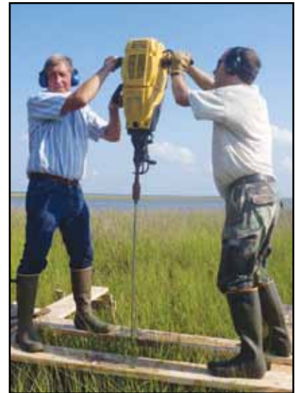
Tom Stadler of the NERR, left, and Philippe Hensel of NOAA install one of 15 surface elevation tables at the Grand Bay NERR.
