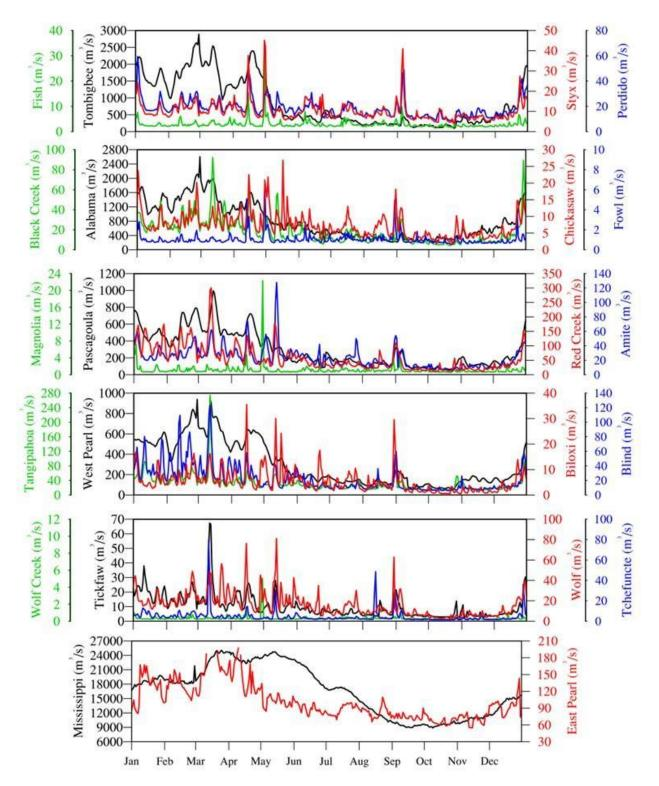
Figure 12. Daily climatology of river discharge (m<sup>3</sup> s<sup>-1</sup>) included in the model for climatological (i.e. typical river discharge) simulations.
