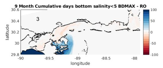
Figure 21. Difference in total cumulative days where average bottom salinity is below 5 (across twin experiments, Table 4) between scenarios with and without active Breton Diversion. Positive values (blue, fresher) indicate there are more cumulative days below 5 in the Breton Diversion scenarios while negative values (red, saltier) indicate there are less cumulative days below 5 in the Breton Diversion scenarios.
