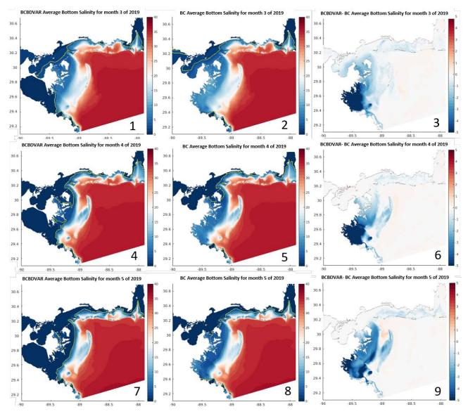
Figure 26. Monthly average bottom salinity for months 3 through 5 of the BCBDVAR (left column) and BC (middle column) cases and the difference across the twin experiment (BCBDVAR-BC, right column). This twin experiment allows for tracking the influence of variable Breton Diversion application when the BCS is active (Table 4). Solid and dashed yellow lines for panels in the left and middle columns track the 2 ppt and 5 ppt isohaline contours, respectively.
