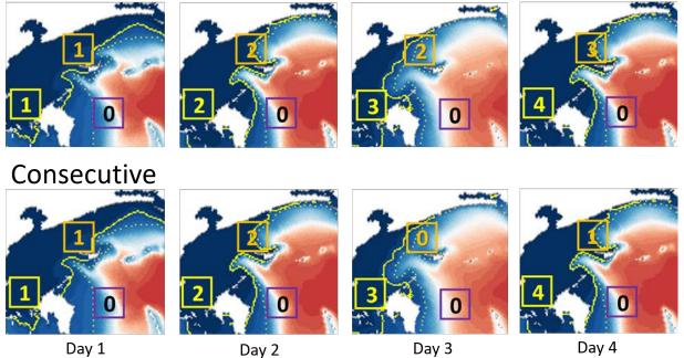
Figure 14-1. Four sequential daily average bottom salinity distributions from the model are shown. The solid and dashed isolines delineate salinity values of 2 ppt and 5 ppt respectively. The numbers in the three box locations illustrate how cumulative time series (top row) and consecutive time series (bottom row) for salinity < 5 ppt are determined for each model grid cell.
